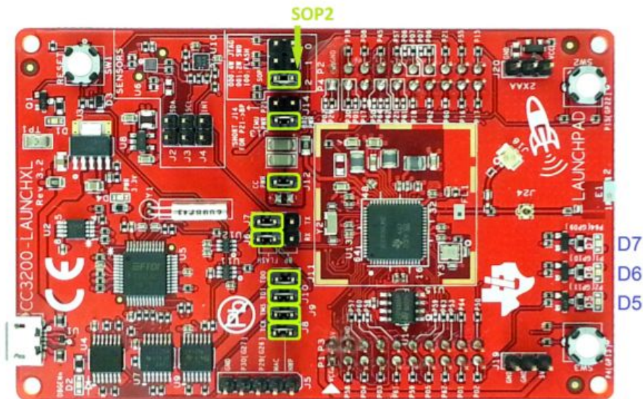
Figure 1. Jumpers on the CC3200-LAUNCHXL
